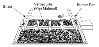
Figure 22 - Fill Entire Burner Pan with Vermiculite
